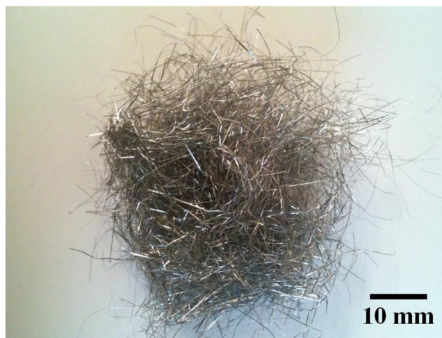
Fig. 1. Photograph of as-cast Ti–Ni fibers fabricated by melt overflow process.
