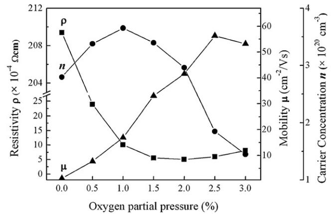
Fig. 2. Variations of the resistivity, mobility and carrier density of IZTO films with different oxygen partial pressures.
