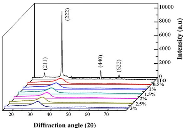
Fig. 1. X-ray diffraction patterns of reference ITO and IZTO films deposited at various oxygen partial pressures on glass substrate.
