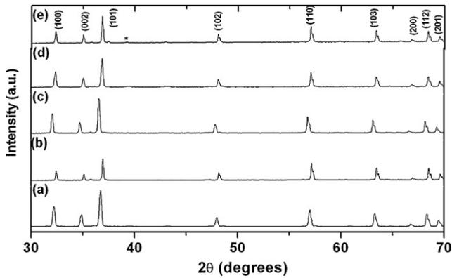
**Fig. 1.** XRD Patterns of polycrystalline  $Zn_{1-x}Co_xO$  system ((a)  $x = 0.00$ ; (b)  $x = 0.03$ ; (c)  $x = 0.05$ ; (d)  $x = 0.07$ ; and (e)  $x = 0.1$ ) (\* indicated the impurity peak of Cobalt oxide).
