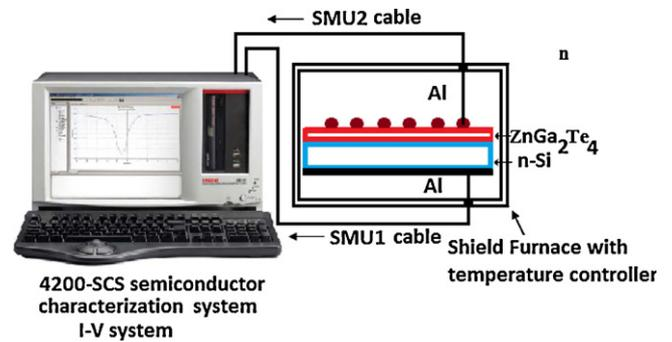
Fig. 1. Schematic diagram of the current–voltage measurement system at different temperatures.
