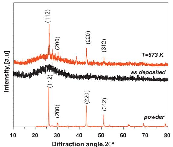
Fig. 2. X-ray diffraction pattern of the  $\text{ZnGa}_2\text{Te}_4$  in powder form, as-deposited thin film and annealed film at 673 K.
