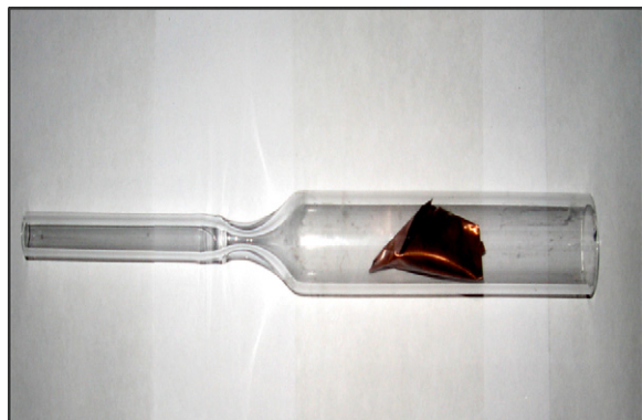
Fig. 1. Photograph of the ampoule used for the synthesis of \text{BaSnF}_4 through solid state reaction.
