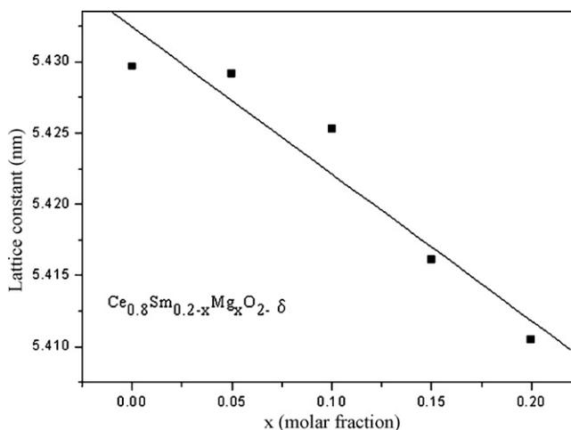
Fig. 2. Relationship of unit cell parameters and dopant concentration of  $\text{Ce}_{0.8}\text{Sm}_{0.2-x}\text{Mg}_x\text{O}_{2-\delta}$ .
