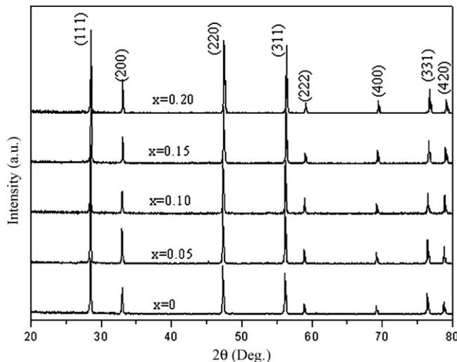
Fig. 1. XRD patterns of  $\text{Ce}_{0.8}\text{Sm}_{0.2-x}\text{Mg}_x\text{O}_{2-\delta}$  sintered at  $1550^\circ\text{C}$ .
