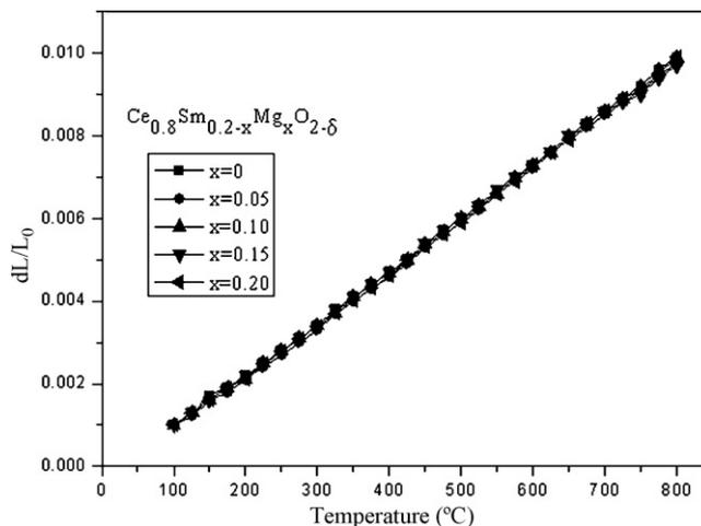
Fig. 3. Linear thermal expansion curves for  $\text{Ce}_{0.8}\text{Sm}_{0.2-x}\text{Mg}_x\text{O}_{2-\delta}$  in air.
