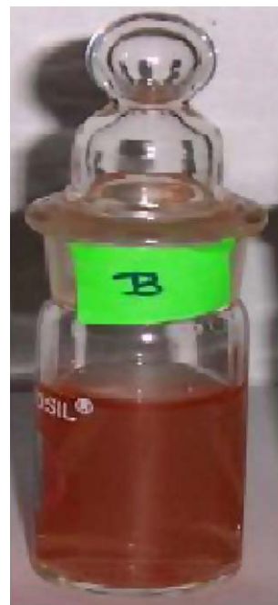
Fig. 1. Aqueous selenium nanoparticles sol obtained by the reaction of 1.0 \times 10^{-3}\text{ mol dm}^{-3} sodium selenosulphate with 1.6 \times 10^{-2}\text{ mol dm}^{-3} acrylamide in the presence of 0.05% PVA.
