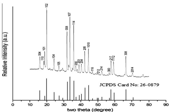
Fig. 1. XRD pattern of  $\text{SrMgAl}_{10}\text{O}_{17}:\text{Eu}^{2+}$  (1 mol%) phosphor.
