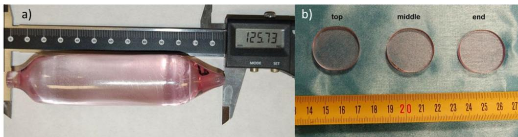
Fig. 1. (a) Ti-sapphire crystal grown by Czochralski technique in ILM. (b) The wafers taken from the different positions of the crystal.
