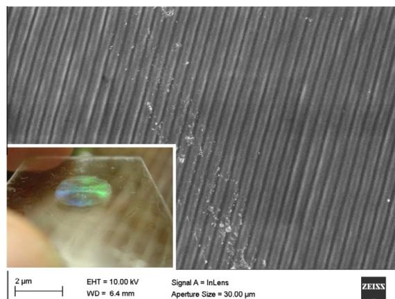
Fig. 3. SEM upper view of the grating structure. The inset shows the sample iridescence (see Experimental Section 2.2).
