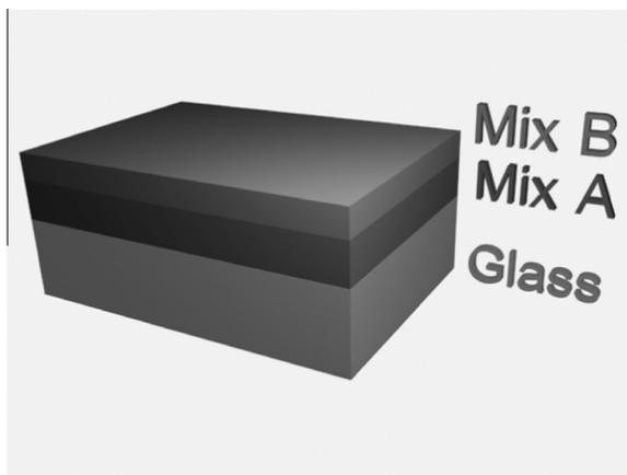
Fig. 1. Schematic view of the sample after the two polymeric layers deposition.
