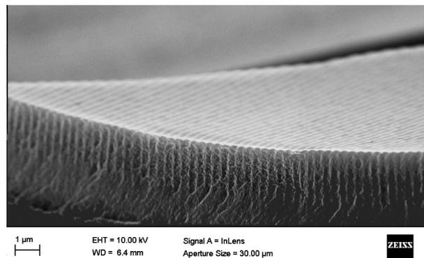
Fig. 2. SEM Cross section of the sample in which the junction between the two substrates is clearly visible.
