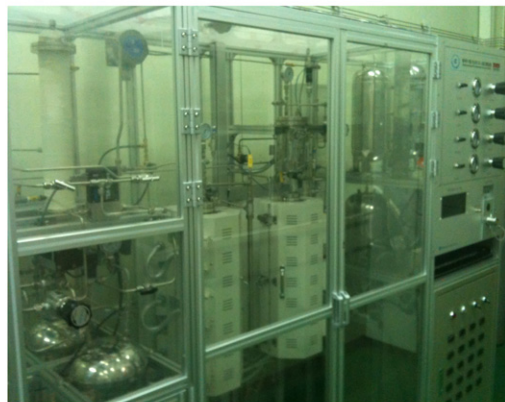
(b) Picture of WGS/multi-layer membrane system
