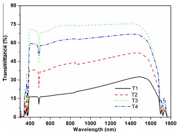
Fig. 3. Optical transmittance of the mirror polished transparent ceramic samples.
