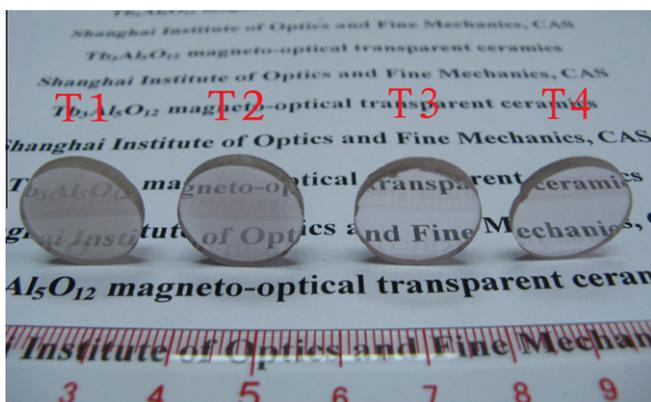
Fig. 1. A picture of the mirror polished ceramic samples.
