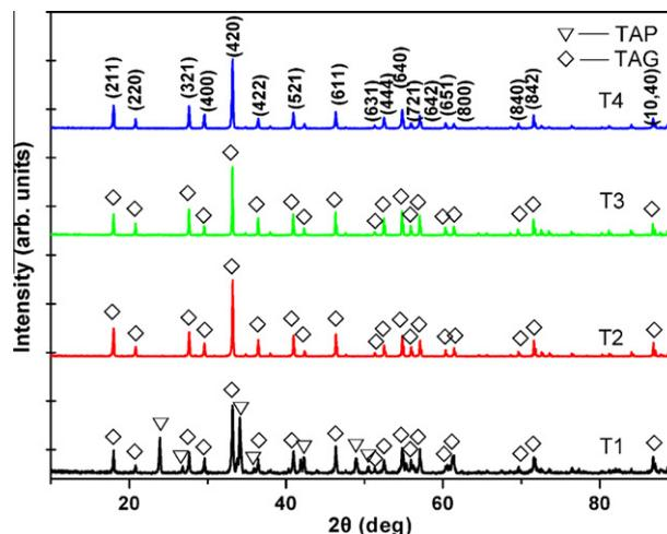
Fig. 2. XRD  $\theta$ - $2\theta$  scans of the four transparent ceramic samples.
