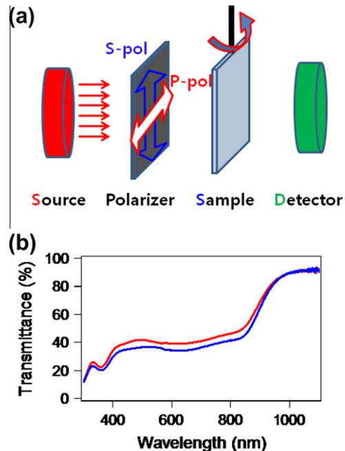
Fig. 1. (a) Schematic showing the modified UV–Vis spectrometer by inserting a polarizer and a rotatable sample holder. (b) The transmittance characteristics of the employed thin film polarizer.
