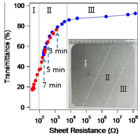
Fig. 2. Transmittance vs. sheet resistance of nickel film deposited on glass by sputtering without rotating the substrates during the deposition for 3 min (blue) and 10 min (red). The inset shows the nickel film deposited on glass for 3 min without rotation of the substrate. (For interpretation of the references to colour in this figure legend, the reader is referred to the web version of this article.)
