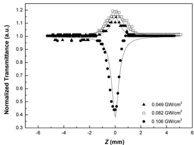
Fig. 2. Relative transmission at 1064 nm and 4 ns pulse duration of the 0.5 at% Sn doped GaSe crystal.
