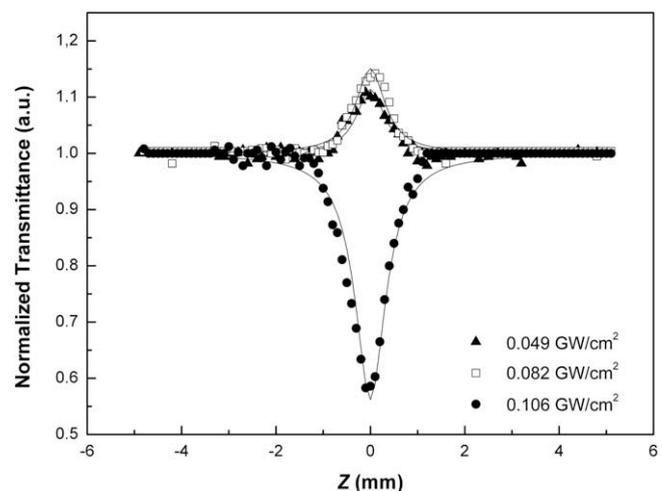
Fig. 3. Relative transmission at 1064 nm and 65 ps pulse duration of the 0.5 at% Sn doped GaSe crystal.
