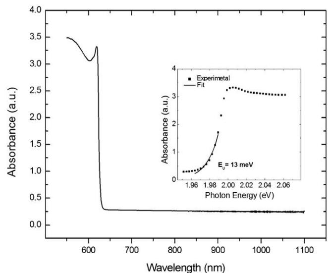
Fig. 1. Linear absorption spectrum of the 0.5 at% Sn doped GaSe crystal. The inset shows the Urbach fit (given as solid line) of the long wavelength tail of the absorption.
