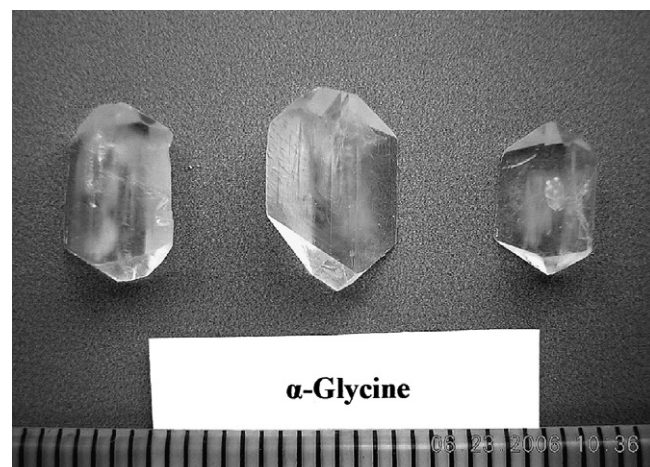
Fig. 3. \alpha -Glycine single crystals resulted from solution with 5 g of NaCl concentration in 100 ml of water.
