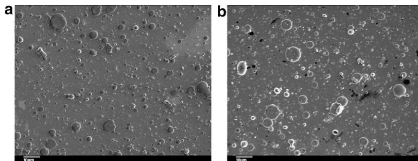
Fig. 1. SEM images of the (a) uncoated and (b) coated phosphor thin films with a magnification of 1000 $\times$ , 10 kV electrons, scale – 10  $\mu\text{m}$ .
