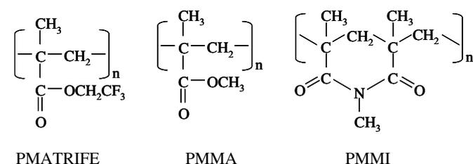
Fig. 1. Cladding polymer PMATRIFE on the left, core polymers PMMA in the middle and PMMI on the right.
