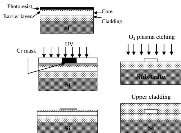
Fig. 2. Scheme of the process for the realization of integrated polymer circuits.
