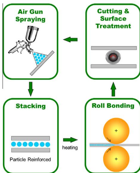
Figure 1. Nanoparticle reinforcement during the ARB process.
