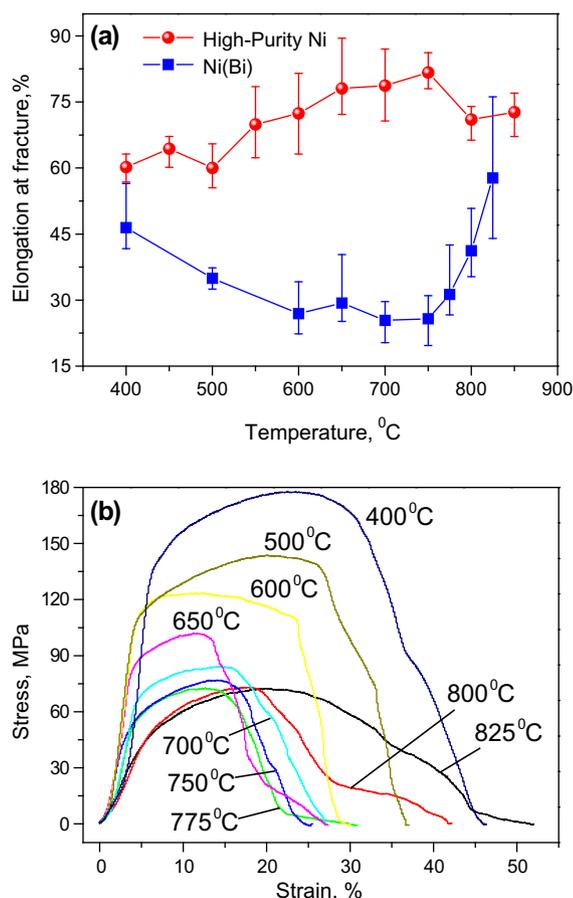
**Figure 1.** (a) Elongations of high-purity Ni and Ni(Bi) alloy at different temperatures and (b) representative stress–strain curves of Ni(Bi) alloy.
