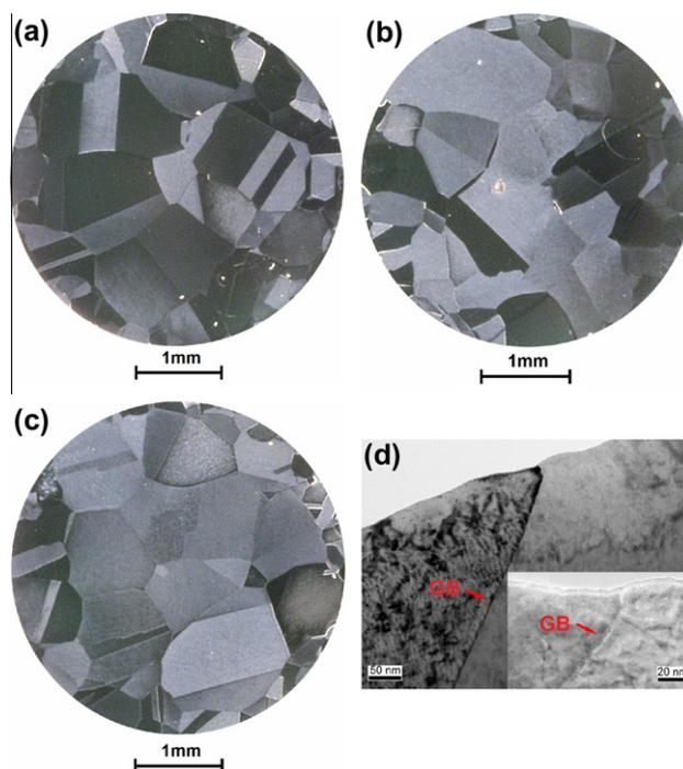
**Figure 2.** Optical microscopy images of samples after tension at (a) 400 °C, (b) 750 °C and (c) 825 °C, as well as (d) a TEM image of samples heat-treated at 750 °C for 45 min.
