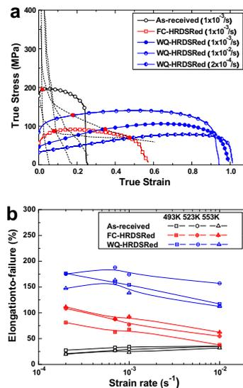
**Figure 1.** (a) True stress–true strain curves of the as-received, FC-HRDSR and WQ-HRDSR 6061 Al at 523 K. The dashed lines represent Hart's necking criterion:  $\sigma = \frac{1}{1-m} \frac{d\sigma}{d\epsilon}$ . The intersection points are indicated by red-filled symbols. (b) Tensile elongation data of the three materials at temperatures 493–553 K given as a function of strain rate.
