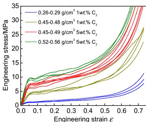
**Figure 2.** Quasi-static compressive stress–strain curves of 1 and 5 wt.% fiber/aluminum composite foams of varying densities.
