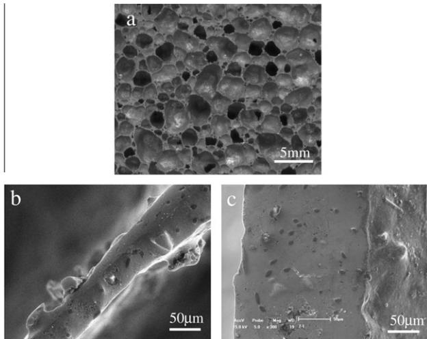
**Figure 1.** Macrostructure and microstructure of closed-cell copper-coated carbon fiber/aluminum composite foam: (a) the present closed-cell foam with 5 wt.% fibers ( $\rho = 0.351 \text{ g cm}^{-3}$ ) Distribution of fibers in the cell wall of foams with (b) 1 wt.% fibers and (c) 5 wt.% fibers.
