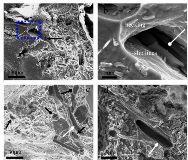
**Figure 3.** Fracture surfaces images of fiber/aluminum composite foam with (a) 1 wt.% fiber and (c) 5 wt.% fiber. (b) Detail of (A) in (a) indicating the plastic deformation of matrix and fiber split. (d) Representative image of fiber pull-out and fiber breakage. Arrow  $\rightarrow$  indicates the extruding ends of the fibers,  $\bullet$  indicates the fiber split,  $\blackrightarrow$  indicates the crack deflection.
