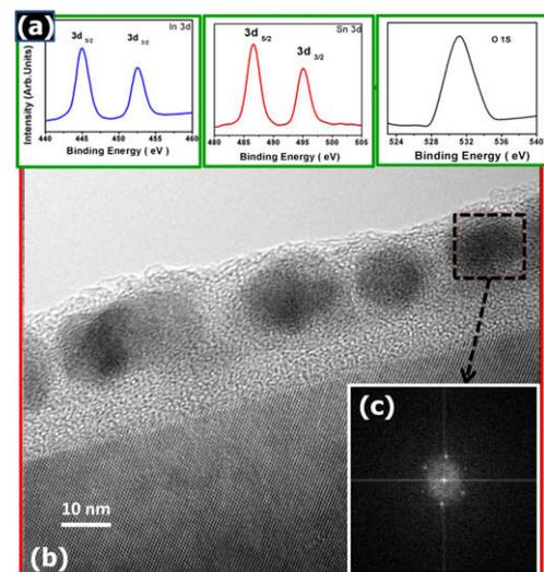
**Figure 2.** (a) Cross-sectional TEM image of ITO films grown at 60 °C; (b) XPS spectra of each element observed in nanoclusters embedded in the ITO films; (c) SADP of ITO nanoclusters.
