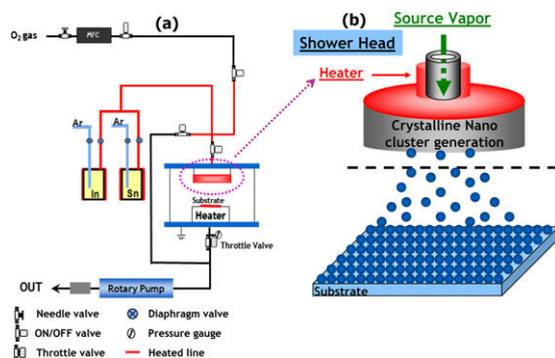
**Figure 1.** (a) Schematic diagram of the NCD method of ITO film growth, and (b) the detailed NCD process occurring at the showerhead.
