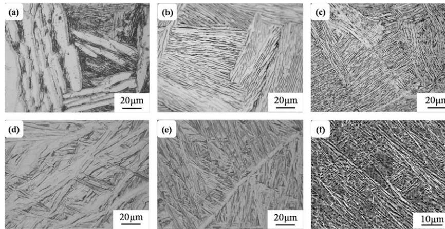
**Figure 1.** Optical micrographs of the initial structure of the alloy prior to deformation processed by (a–c) furnace cooling at 1108, 1073 and 948 K, and (d–f) quench and reheating at 1108, 1073 and 948 K, respectively.
