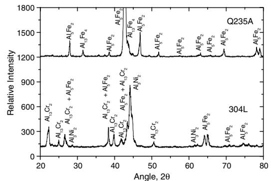
**Figure 3.** X-ray diffraction pattern of the diffusion layers of the Q235A and 304L.
