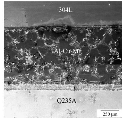
**Figure 2.** Microstructure of the 304L/Al–Cu–Mg/Q235A sample cladding at 640 °C for 20 min.
