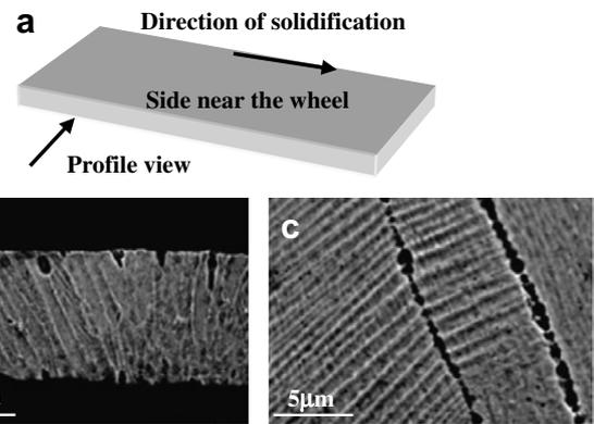
Figure 2. (a) Sketch map of the ribbon, (b) BSE micrographs of the  $\text{Ni}_{50}\text{Mn}_{36}\text{In}_{14}$  ribbon profile view and (c) martensitic stripes on the profile of the ribbon.
