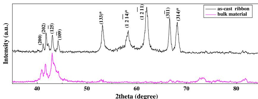
Figure 1. XRD of the  $\text{Ni}_{50}\text{Mn}_{36}\text{In}_{14}$  bulk material and ribbon as-cast in room temperature.
