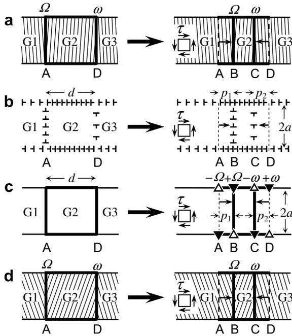
**Figure 1.** Geometric (a, d), dislocation (b) and disclination (c) models for stress-induced cooperative migration of two low-angle (a, b) or high-angle (c, d) grain boundaries under an external shear stress  $\tau$ .
