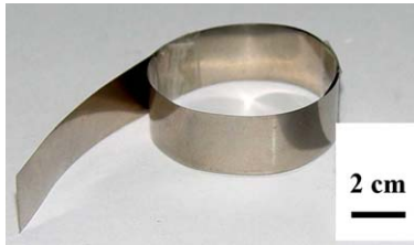
Figure 1. Optical photograph of Ni 3 Al foil with a thickness of 300 μm obtained by rolling at LN 2 T to 95% of CW.
