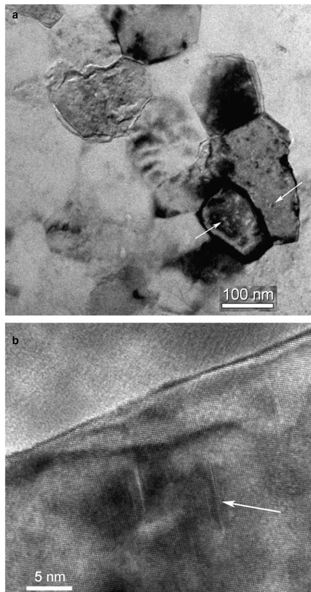
Fig. 1. Microstructure of the as-extruded cryomilled 5083 Al alloy in a section normal to the extrusion direction.
