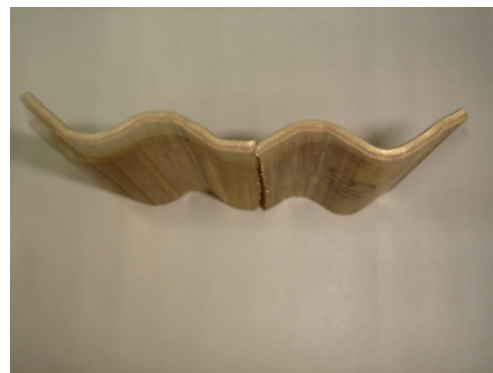
Figure 2. A cracked Cu-38Zn sheet after two pressing cycles. Note that cracking occurs at the corner of the groove pressing tooth.
