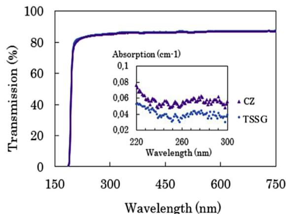
Fig. 2. Transmission curves for CZ and TSSG crystals; inset: absorption curves near 257 nm for TSSG (blue circles) and CZ (purple triangles). (For interpretation of the references to color in this figure legend, the reader is referred to the web version of this article.)
