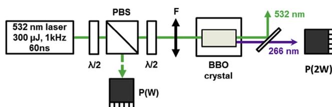
Fig. 3. Experimental setup for SHG.
