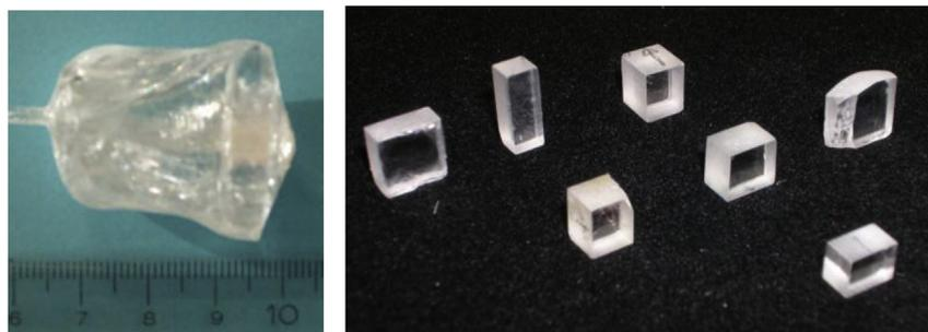
Fig. 1. Czochralski  $\beta$ -BBO grown in super cooled melt (left). Samples are sawn from clear and less stress part of the bowl. Oriented and polished sample (right).
