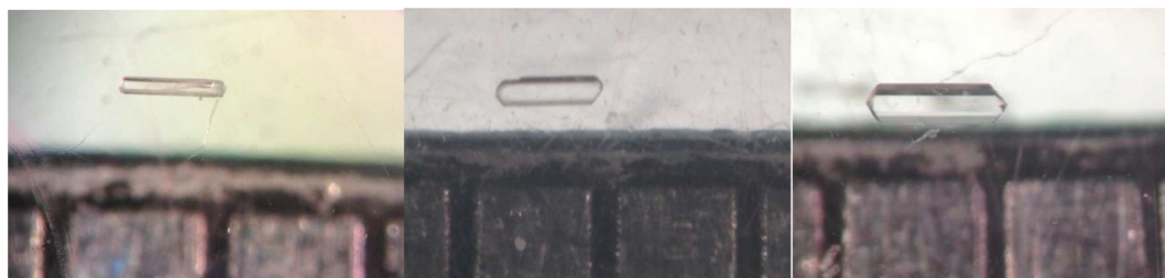
Fig. 1. Crystal images of the average size of Na 5 Er(OH) 6 WO 4 (left), Na 5 Yb(OH) 6 WO 4 (center), and Na 5 Tm(OH) 6 WO 4 (right) crystals where the scale bar below the crystals denotes mm increments.
