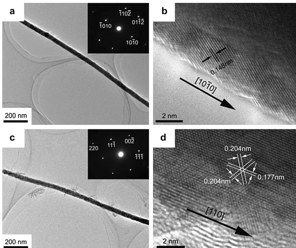
**Fig. 1.** TEM and HRTEM images of Co nanowires with different structures: (a) TEM image of hcp Co nanowire and SAED pattern, (b) HRTEM image corresponding to the nanowire shown in (a), (c) TEM image of fcc Co nanowire and SAED pattern, (d) HRTEM image corresponding to the nanowire shown in (c).
