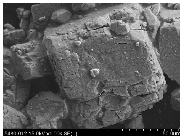
Fig. 3. SEM image of self-organized H_5PV_2Mo_{10}O_{40} material.
