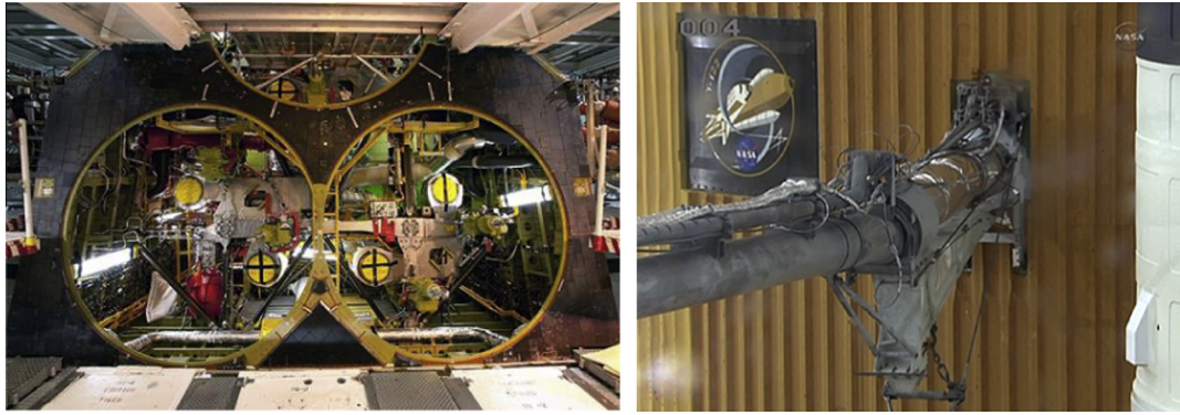
Fig. 1. Examples of piping complexity in aerospace cryofuel systems: the aft compartment of the Space Shuttle Orbiter Discovery with its main engines removed (left) and the Shuttle External Tank LH 2 Vent Umbilical (right).
