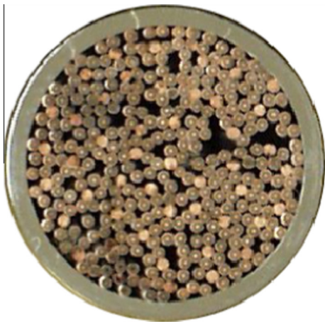
Fig. 2. CICC conductor [2] used in the hot-spot experiment. The original 1 mm thick steel jacket shown on the photograph was replaced by a 10 mm thick one.
