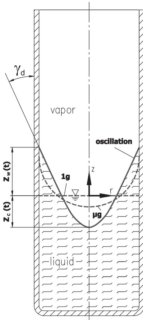
**Fig. 1.** Sketch of a generic experimental cell for the investigation of the reorientation with characteristic values of the oscillation, the contact line coordinate on the wall  $Z_w(t)$  and the center coordinate  $Z_c(t)$ . The angle between the interface and the wall at the position of the contact line is the dynamic contact angle  $\gamma_d$ .
