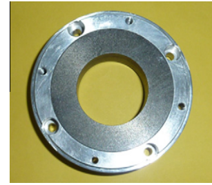
Fig. 3. One of the \text{GdBa}_2\text{Cu}_3\text{O}_7 ring bulk superconductors used in Magnet B.
