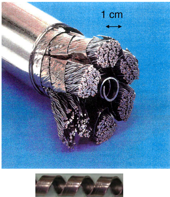
Fig. 1. A typical ITER CICC (top) and the spiral delimiting its central channel (bottom).
