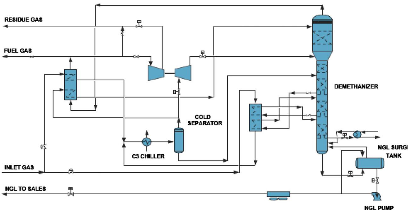
Fig. 1. Process flow diagram for a turboexpansion-based NGL production plant.
