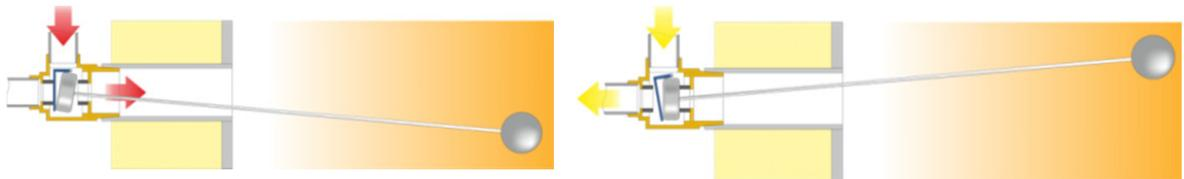
Fig. 2. Graphic depiction of how the Thermo-Differential Valve switches the flow based on temperature difference with the storage tank.
