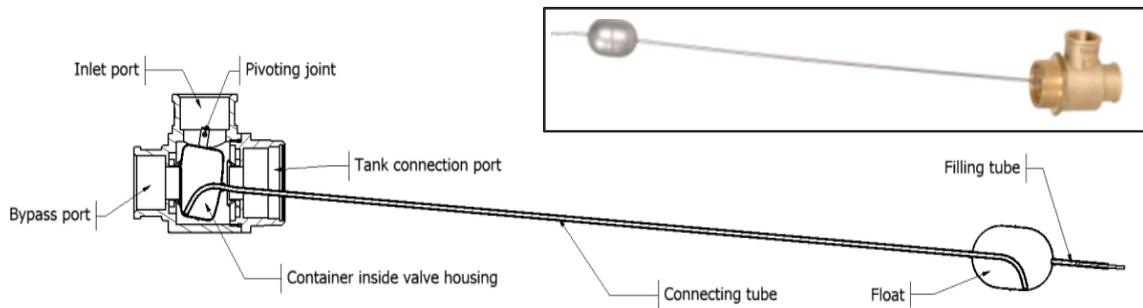
Fig. 1. Cross-section drawing of the Thermo-Differential Valve, and an inset picture of the Thermo-Differential Valve
