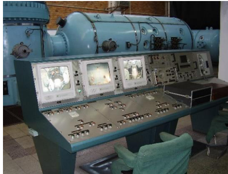
Fig. 1. The diving chamber and the associated control panel owned by the Dive Center of Constanța
