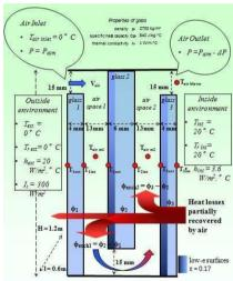
Fig. 1: Data and boundary conditions
