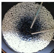
Fig 1. A photograph of ceria coated foam device under the thermal reduction step
