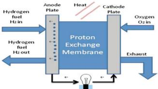
Fig. 1. Diagram of Fuel Cell Operation.
