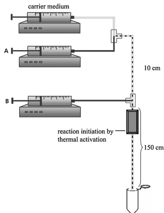
Fig. 1. General set-up for micro segmented flow synthesis of bimetallic multishell nanoparticles.
