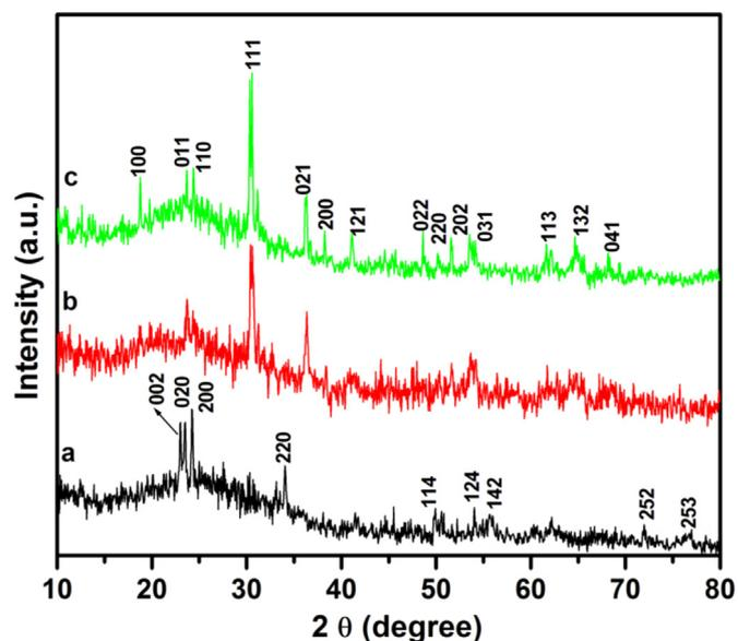
Fig. 2. XRD patterns of (a) as-prepared sample ( $\text{Zn-WO}_3$ ), (b) sample heat treated at 400 °C for 2 h and (c) sample heat treated at 500 °C for 2 h.
