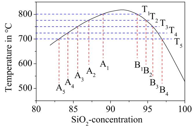
Fig. 1. Binodal metastable phase diagram in the system  $\text{Na}_2\text{O}$ – $\text{SiO}_2$ . At the temperature  $T_1$ , liquid phases with the compositions  $A_1$  and  $B_1$  are formed.
