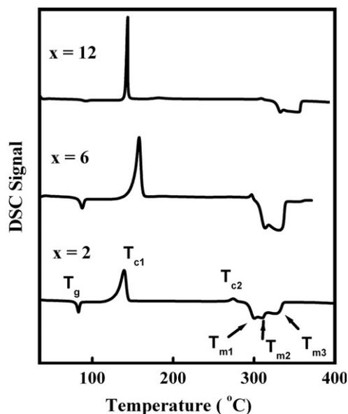
Fig. 2. DSC thermograms of the  $\text{Se}_{60-x}\text{Te}_{40}\text{Sb}_x$  glasses recorded at a heating rate of 10 °C/min for representative compositions ( $x=2, 6$ , and 12).
