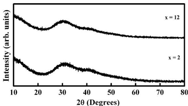
Fig. 1. XRD patterns of the representative samples ( $x=2$  and 12) showing the amorphous nature of the prepared samples.
