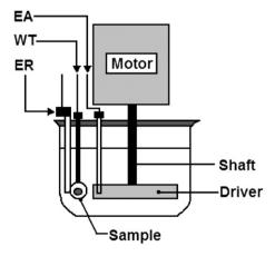
**Fig. 1.** Schematic diagram of the device used at corrosion–erosion wear testing. Auxiliary electrode (EA), working electrode (WT), reference electrode (ER) were used in the test [13].
