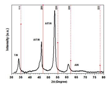
**Fig. 2.** XRD patterns for TiN/AlTiN multilayered grown with  $\Lambda\!=\!250\,\mathrm{nm}$ . Dash lines indicate the position of the peaks obtained from JCPDF 462553 files from ICDD cards.
