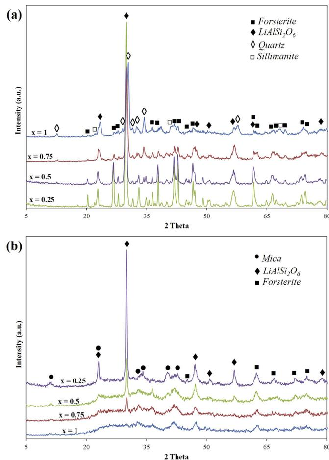
Fig. 1. XRD patterns of the samples heat treated at  $700^\circ\text{C}$  for 4 h and prepared in different  $x$  values based on (a)  $\text{Li}_{(1+x)}\text{Mg}_3\text{AlSi}_3(1+x)\text{O}_{10+6.5x}\text{F}_2$  and (b)  $\text{LiMg}_3\text{AlSi}_3(1+x)\text{O}_{10+6x}\text{F}_2$  compositions.
